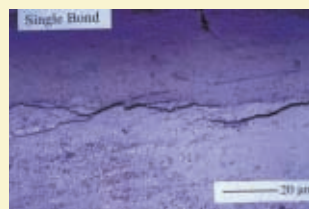
Figure 9 Laser scanning microscopic image of the bonding interface between enamel and Single Bond showing the crack propagation along the prisms under the interface.
