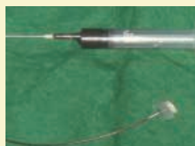
Figure 11 The occlusal surface was ground and the root was also removed. The crown segment was bonded to a plastic plate and connected to a syringe to be able to apply a pressure from pulpal side. The pulp chamber was filled with a red dye solution.
