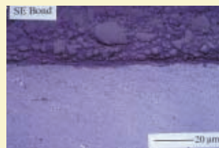
Figure 10 Laser scanning microscopic image of the bonding interface between enamel and SE Bond showing the tight bonding without crack propagation.
